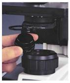
40X phase Contrast Attachment (Simple plug in type)
